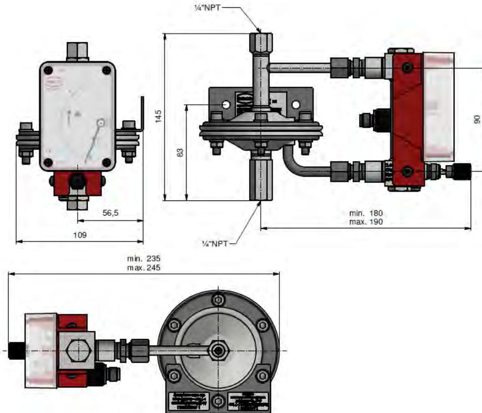
10.4 KDS-R with 1/4" NPT (F) connection as inlet pressure regulator version
