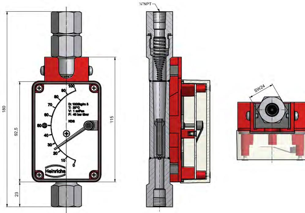
**10.3 KDS-R with 1/4" NPT (F) connection as outlet pressure regulator version**
