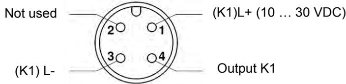
**12.2.5 M12 standard configuration 2 x inductive sensors NBB 2-6.5M 30-E2**
