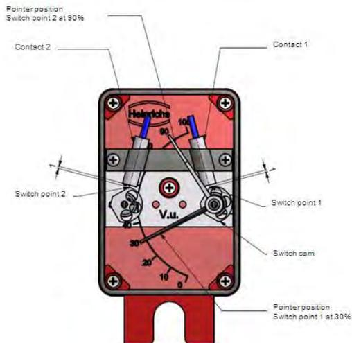
Set pointer to the desired switch point and adjust scale. Turn up switch cam so that the edge of the switch cam is located in the center of the diameter of the proximity switch
