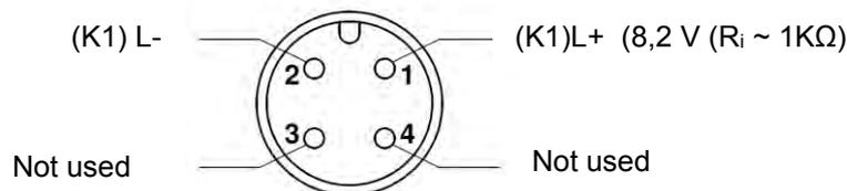
**12.2.4 M12 standard configuration 1 x inductive sensor NBB 2-6.5M 30-E2**
