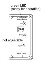
The instrument is delivered ready to operate. The electronics are matched and calibrated against the signal transmitter. The calibration screws ('ZERO' and 'RANGE') found behind the adhesive foil must not be adjusted by the customer. If they are adjusted, a re-calibration will be required involving new calculations. Should the electronics be opened, any warranty will become invalid.
