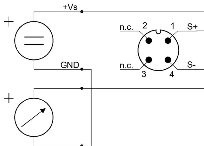
2-wire, DIN plug connector (..L442)
