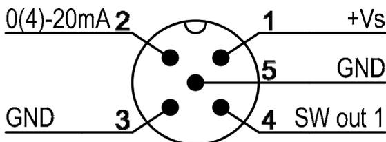
The clamps 3 and 5 are short-circuited and can therefore be used optional for the output signal or power supply.
