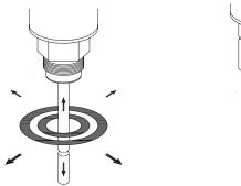
Single Rod/Rope Probe Application Area
