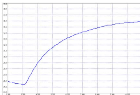
Signal graph without Smart Averaging function
