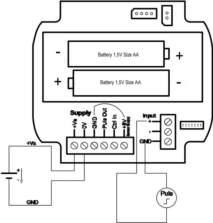
Wiring for ZOE-Z with Supply option B:
