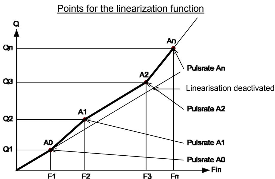
With active linearization function, the number of linearization points for parameter „linearization points“(in addition to point A0) is set fixed. Depending on the setting of this parameter, the other input parameters are shown in the menu. Input signals above the last point linearization are processed with the pulse rate of the last point.
