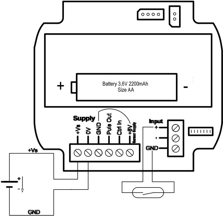
Wiring for ZOE-Z with Supply option B:
