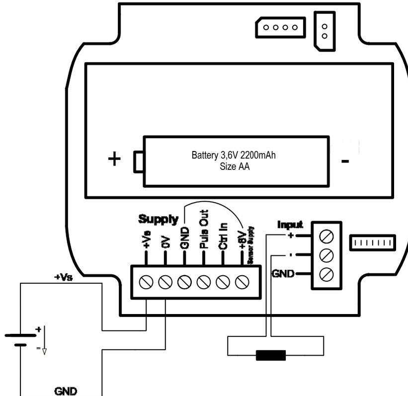
The connection of the DOT (turbine wheel flowmeter) is identical to the connection of the induction coil.
