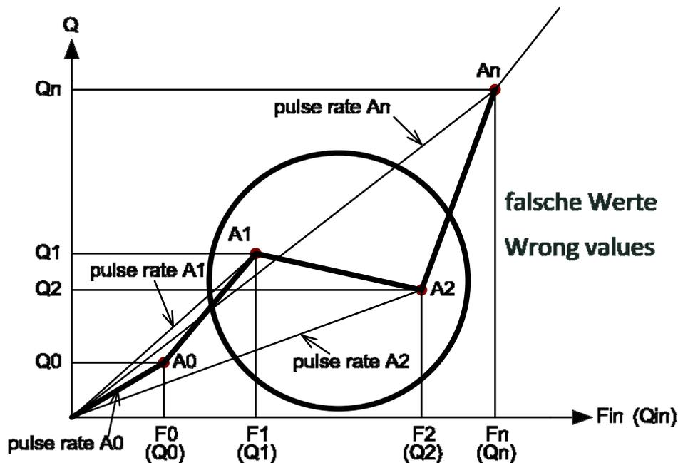
To correct this error, the bases must be checked and corrected if necessary. This must always apply:
